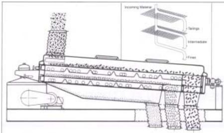
Flow diagram showing typical two-surface FIOTEX Screener
